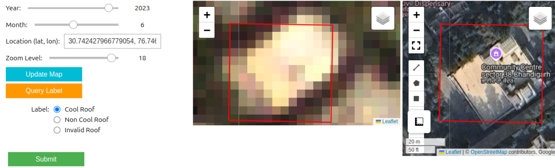
Fig. 3. The annotation dashboard interface displaying Google Maps[9] and Sentinel-2 RGB Bands imagery [8] with roof squares bounding box to polygon mapping for guided labelling.
