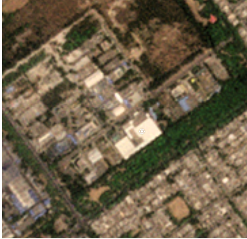
Fig. 9. Illustration of an area where the expected cooling effect of cool roofs is not observed due to surrounding vegetation and a high density of cool roofs within the 100-meter radius.
