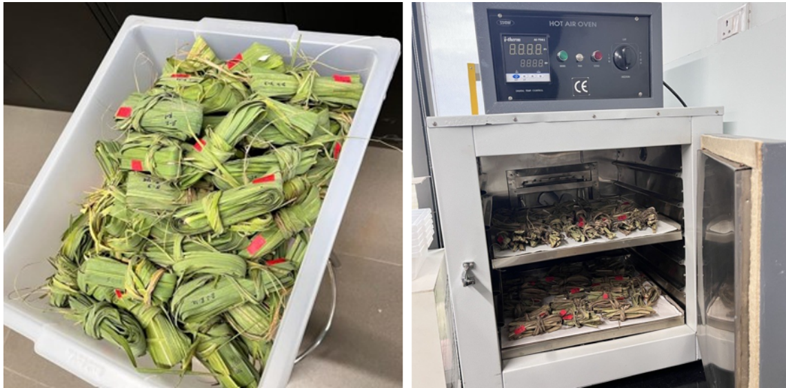
Fig. 4. Leaf samples collected from the farm are stored in a box to preserve moisture (left). Within 24 hours, leaf samples are dried in an oven (right). Weights are taken at both stages to estimate leaf water content.
